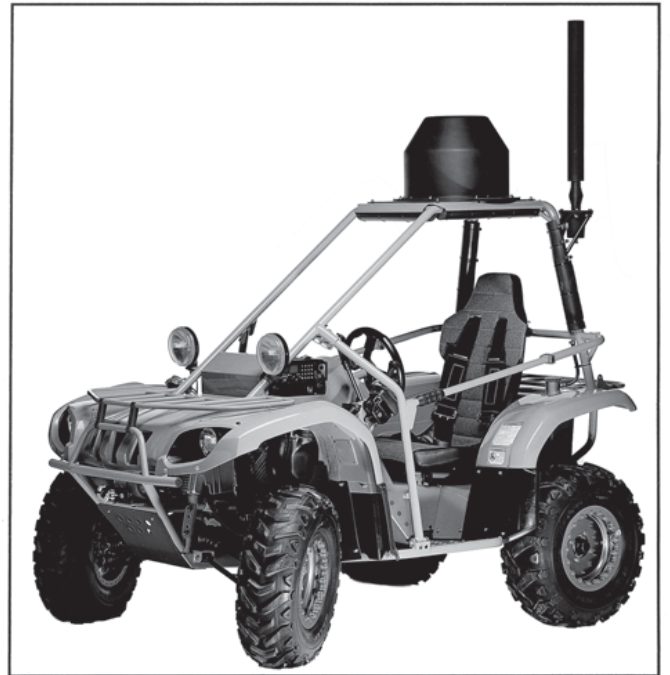
Figure 4. The Prowler RTV is available in two platforms: Light Surveillance, Recon and Communications (shown) and Light Weapons/Reconnaissance. All Terrain Vehicle
